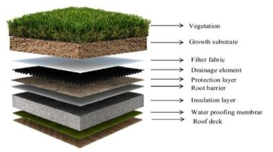
Typical components of a green roof.
